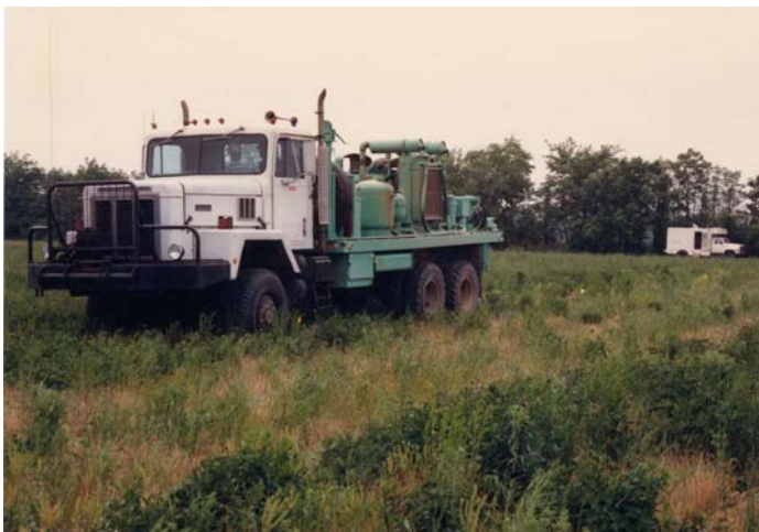
Since the 1980s, Gochioco successfully used the Conoco high-frequency Vibroseis as a seismic source in shallow geophysical investigations. Recording truck is located in the background. It took nearly 12 years later before other geophysicists worldwide learned how to use this source type in near-surface geophysics surveys (circa 1987).
