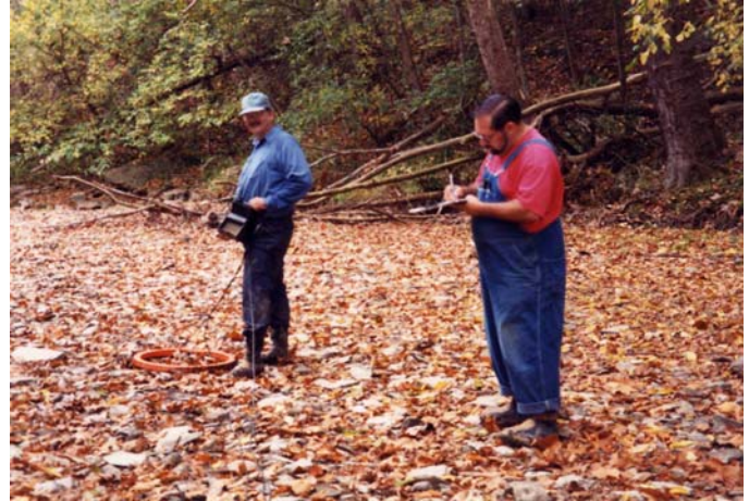
Fred Ruev occasionally supervised some field projects - an electromagnetic (EM) survey on a dry streambed.
