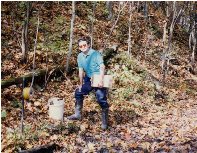
An electrical resistivity survey along a stream bank.
